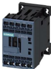
Power contactor, AC-3 16 A, 7.5 kW / 400 V 1 NO, 24 V DC 3-pole, Size S00 Spring-type terminals
